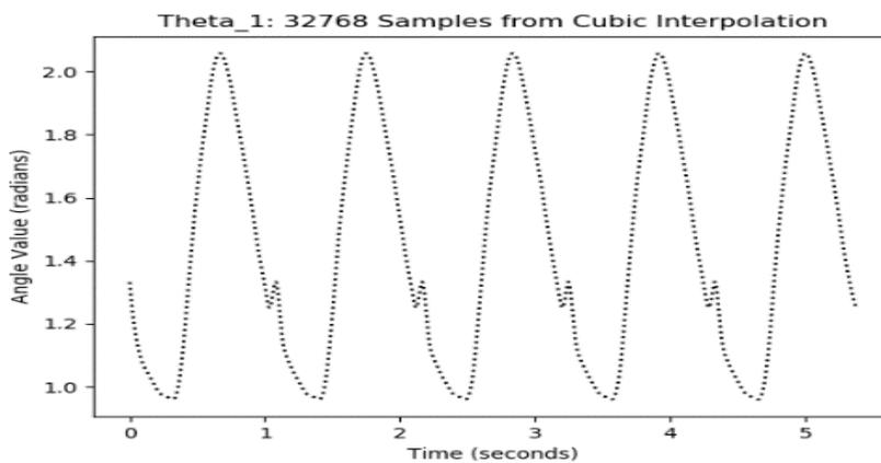
Fig 9(c): Optimized Motion curve of Right Shoulder Joint of a tiger during the walk
