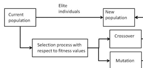
Fig 8: Genetic Algorithm based optimization scheme (source: [8])
