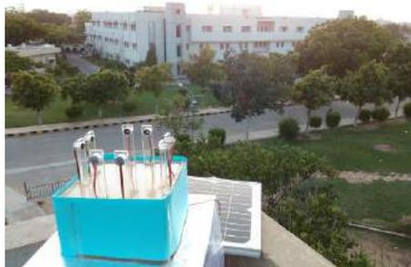
Figure 4: Testbed deployment of advance version of ultrasonic anemometer
