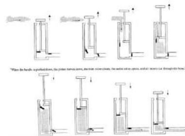
**Figure 4:** Selected animation frames and corresponding narration from a multimedia lesson on how a tire pump Works [8] [11].
